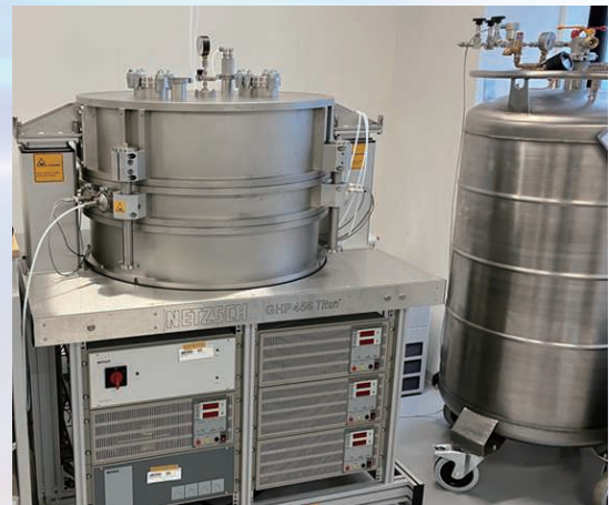
Cryogenic thermal conductivity measuring device
