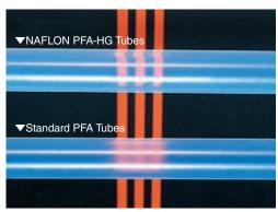
\* Photo to compare transparency between NAFLON™ PFA-HG Tube and standard PFA Tube (Our products' comparison)
